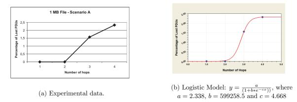
Figure 5: a) Relation between the percentage of lost PDUs and the number of hops. b) The analytical function representing the relation observed in the experimental data.
