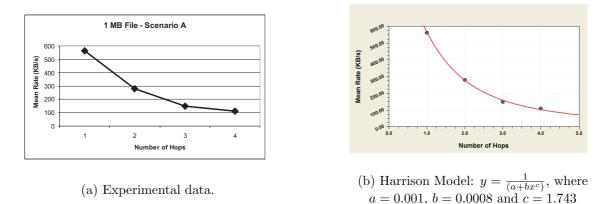
Figure 4: a) Relation between the mean data rate per download and the number of hops. b) The analytical function representing the relation observed in the experimental data.
